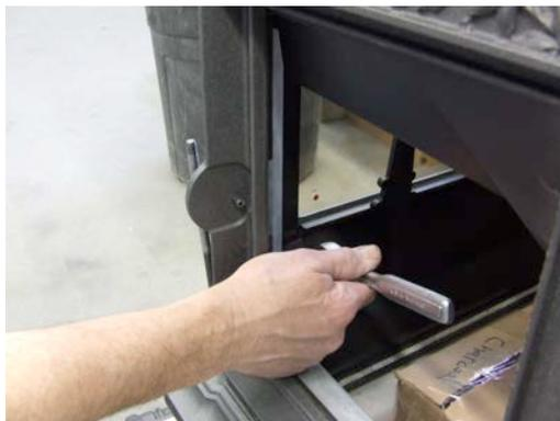
8. Hold the stone over the door securely while removing the door frame. Pull the top of the frame out away from the stove body and off of the stove base. Once the frame has been removed, slide the stone out from under the rope.
