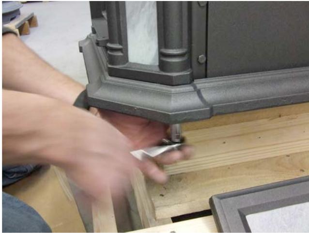
6. Remove the cast iron corners by lifting them up and swinging the bottom edge away from the stove. Slide the corners out from under the rope.
