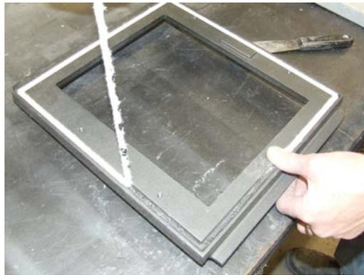
10. Use a small bead of gasket glue in the gasket channel, then start the .375" gasket slightly offset from the center, at the bottom of the door frame.
