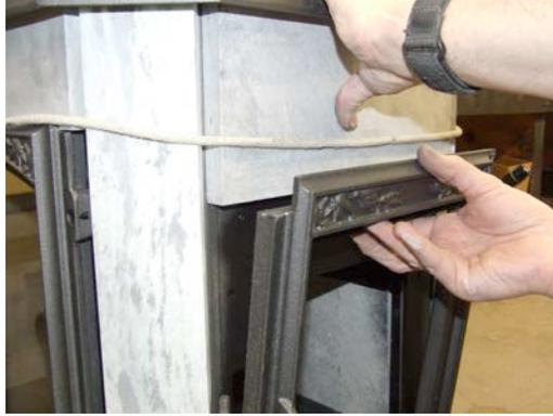
9. Lay the frame face down on a flat surface. Pull the old gasket out of the channel in the frame. Use a putty knife or wire brush to clean any leftover gasket or residue from the channel. Brush off or vacuum the gasket channel.
