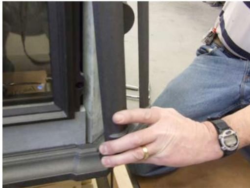
7. The door frame is secured to the steel body box with four bolts from the inside. The top front and bottom rear bolts are  $\frac{3}{4}$ " long and also hold the corner stone retainers. Remove all four bolts with a  $\frac{7}{16}$ " socket.
