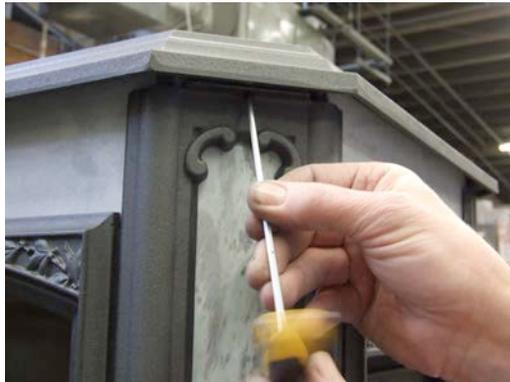
20. Insert the hinge pin in the bottom of the door. Slide the washer over the end of the pin and hold it in place as you set the pin into the door frame. Insert the top hinge pin down through the door frame and into the door.
