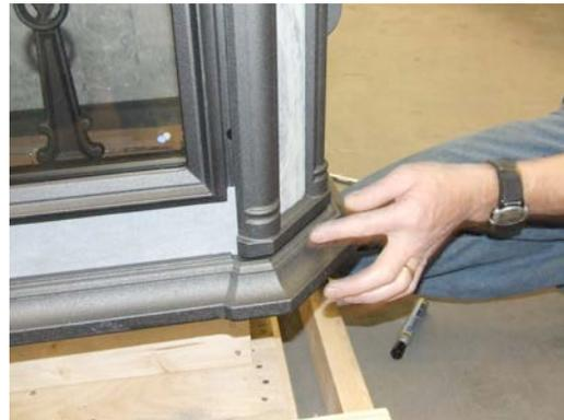
15. Hold the draw rod with your finger near the top and start the nut on the bottom end. Start the nuts on both the front and rear draw rods. Make about (5)  $\frac{1}{4}$  turns with a  $\frac{1}{2}$ " socket on the front nut.
