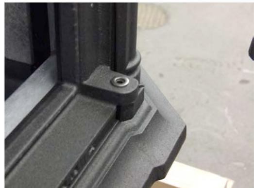
3. Use a 1/8" allen key to loosen the set screws at the top of the front and rear corners adjacent to the door frame.
