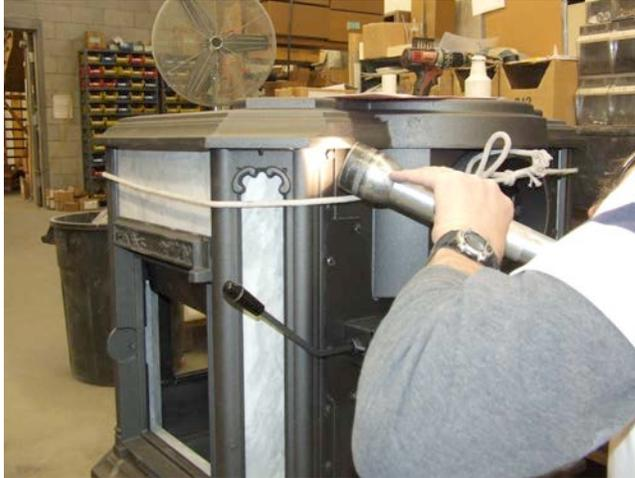
17. Gently tighten the rear draw until the top cast contacts the pin in the body box. Do not over tighten and bend the pin.
