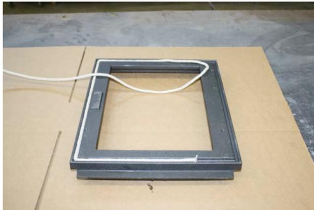
11. Take the flat adhesive gasket and apply it to the inner perimeter of the door frame, as shown below.
